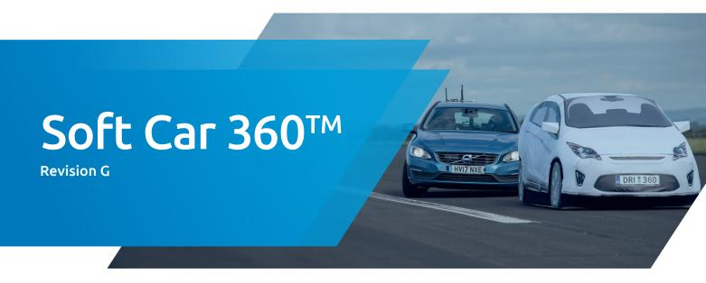
Soft Car 360 from DRI is a lightweight, durable vehicle target which forms the perfect ADAS testing solution when combined with AB Dynamics' GST Platform. With the proven ability to perform the LSS test at a closing speed of 144kph, causing no damage to the test vehicle, the Soft Car 360 has been specifically adopted as the Global Vehicle Target (GVT) for the Euro NCAP 2020 ADAS tests.
