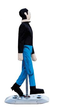
The Soft Pedestrian 360 from DRI is the next generation of articulated surrogate pedestrian target, bringing a whole new level of realism and vehicle protection to VRU testing.
